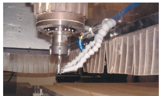
Fig. C. Cold air from EXAIR's Model 5315 Cold Gun System keeps the tooling cool.
